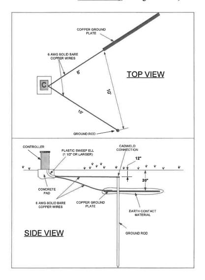
Ground rods are to have a minimum diameter of 5/8" and a minimum length of 10 feet. These are to be driven into the ground in a vertical position or an oblique angle not to exceed 45 degrees at a location 10 feet from the electronic equipment, the ground plate, or the wires and cables connected to said equipment, as shown in the detail above. The rod is to be stamped with the UL logo [Paige Electric part number 182007.] A 6 AWG solid bare copper wire (about 12 feet long)
